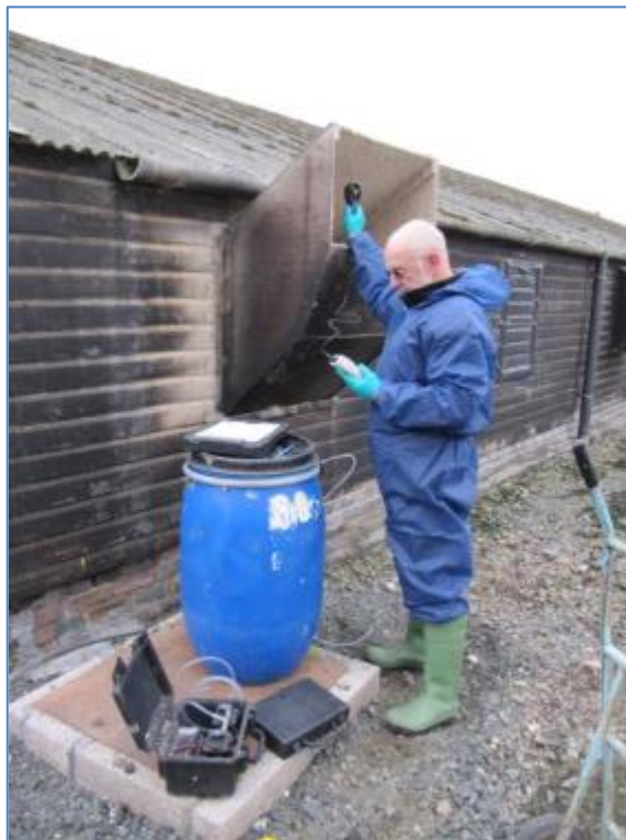
Figure H - 8: Monitoring odour concentrations and fan ventilation flows in the exhaust of Glendevon farm.
