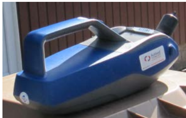
Figure H - 15: DUSTTRAK II ambient particle monitor shown with the PM_{10} size selective inlet in place.
