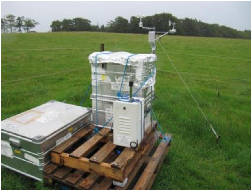
Figure H - 14: Osiris monitor deployed in the field in a weather proof enclosure at Whitelees farm (site White 1).
