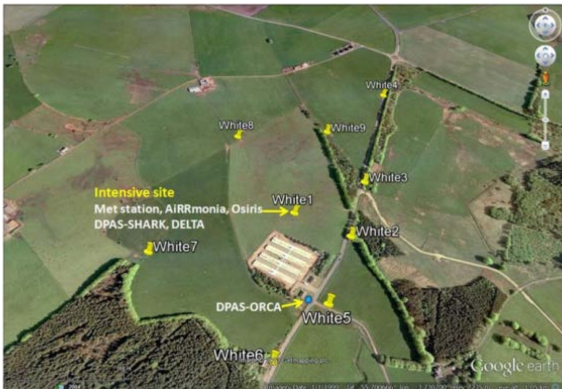
Figure H - 3: Google earth map of the Whitelees Poultry Farm study area, showing the locations of ammonia monitoring sites. White 1 is also the location of the meteorological and intensive (continuous) measurement site.
